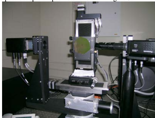
Figure 5: Variable Angle Spectroscopic Ellipsometer with full hexagon wafer mounted for analysis.
